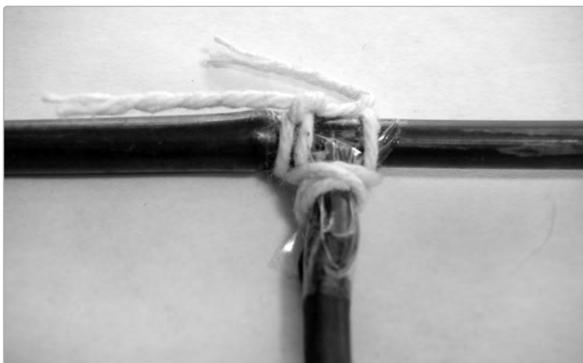
FIGURE 23-18: Wrap the cross braces' joints with string.
