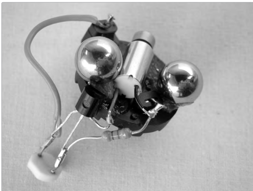
FIGURE 22-10: The resistor connecting the motor to ground and completing the Jitterbug's brain circuit
