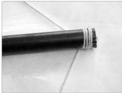
FIGURE 23-9: Detail of the string wrapping at the end of a spar (back side at left; sail side at right)
