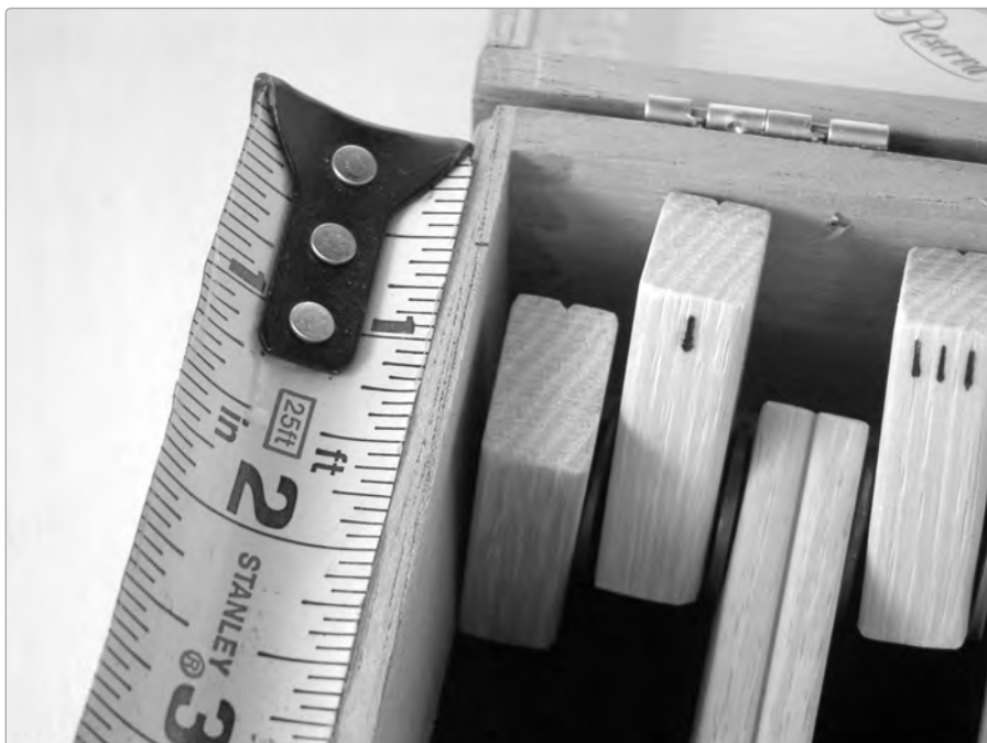
FIGURE 6-7: Measuring the clearance for the scoring tiles
