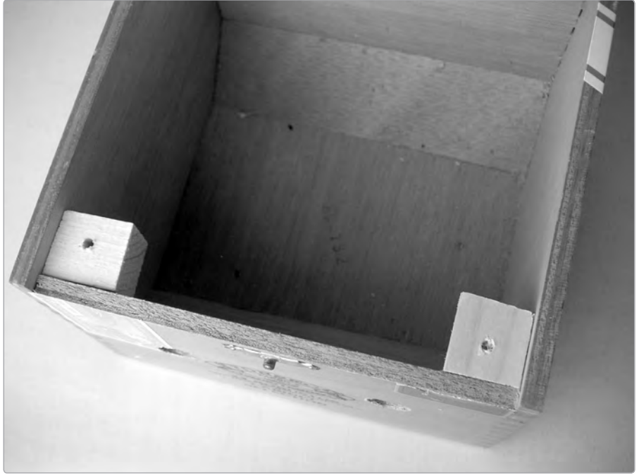
FIGURE 2-4: The blocks installed, with guide holes drilled
