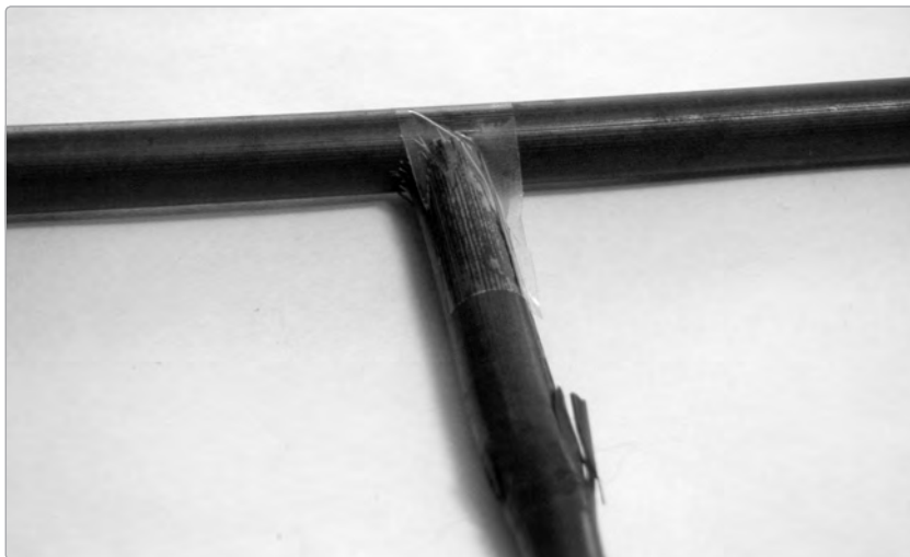
FIGURE 23-17: Secure the cross braces with tape.
