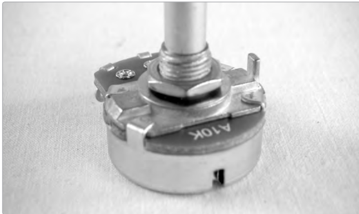
FIGURE 17-12: A close-up of a potentiometer's anchor
