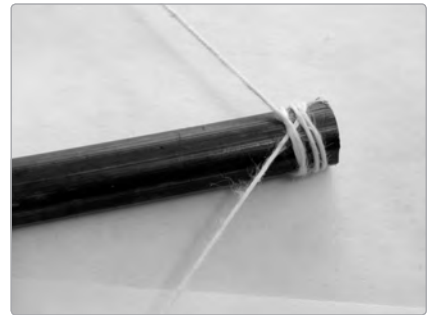
FIGURE 23-9: Detail of the string wrapping at the end of a spar (back side at left; sail side at right)
