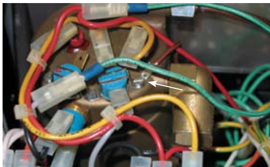
Fig. 1 Thermocouple washer installed under screw of steam thermostat.
