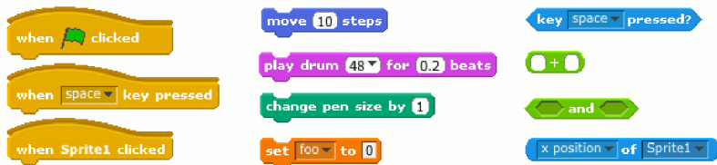
Figure 6-2. There are three types of blocks in Scratch: hat blocks (left), stackable blocks (center), and reporter blocks (right)
