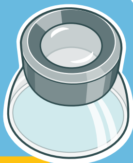
D. LOUPE: Good for checking solder connections on the PCB.
