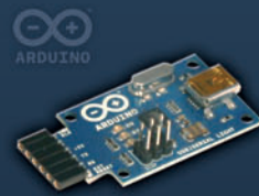
Serial Converter MCM Part #83-14699
