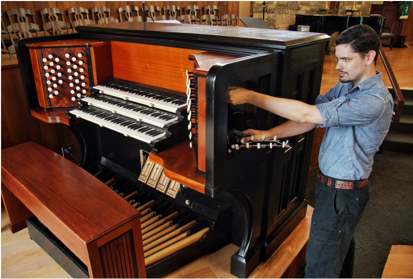
Figure 7-5. Bradley Gawthrop works on electrical cabling for an organ he built in Boone, NC (photo courtesy of Bradley Gawthrop)
