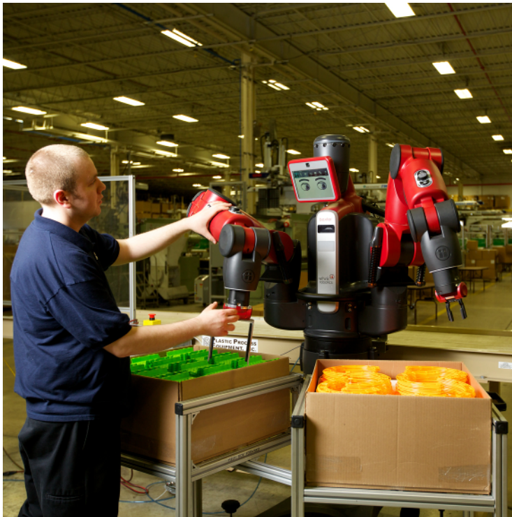
Figure 4-1. The Baxter industrial and research robot scales its movements to human speed, so it's safer to work around. Credit: Rethink Robotics.
