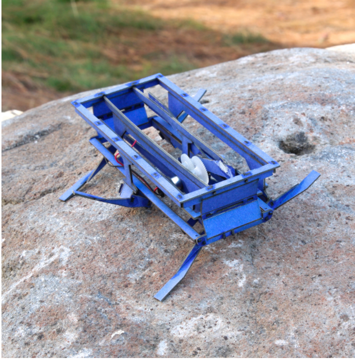
Figure 1-4. Dash is a robotic bug made from laser-cut cardboard and easily assembled. Credit: Dash Robotics.
