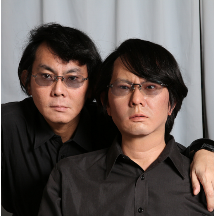
Figure 4-8. Hiroshi Ishiguro developed Geminoid HI-4 in his own image to explore whether human presence could be transferred to a remote location using robots. Credit: Hiroshi Ishiguro, Osaka University.
