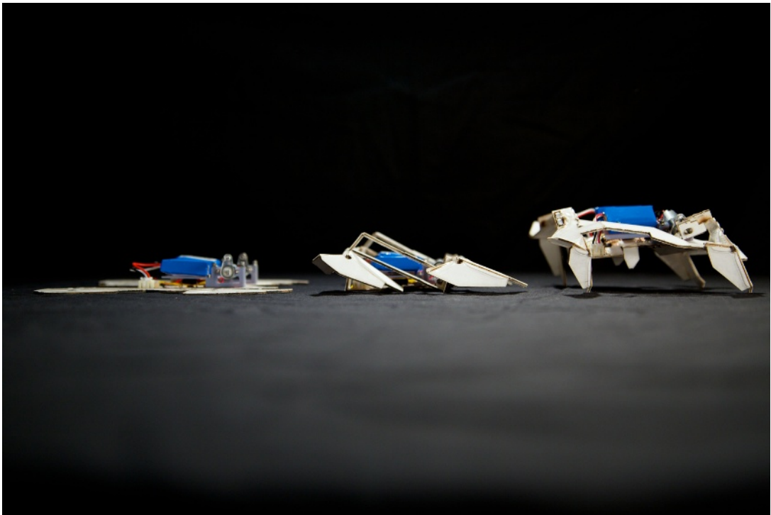
Figure 1-2. This robot made of paper and heat-activated shape memory polymer from Harvard and MIT scientists can fold itself up and scurry away. Credit: Seth Kroll/Harvard's Wyss Institute.
