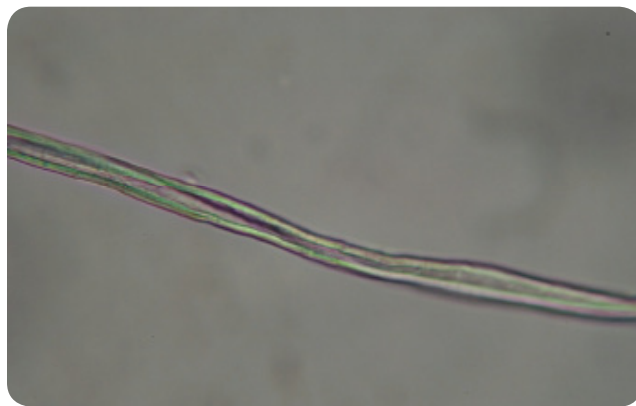
Figure II-7-12: As focus is opened, the Becke line moves toward the center of the fiber
