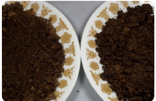
Figure I-1-4: Soil specimens before (right) and after drying
