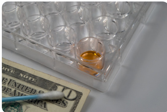
Figure VII-2-2: A positive Marquis reagent test for methamphetamine
