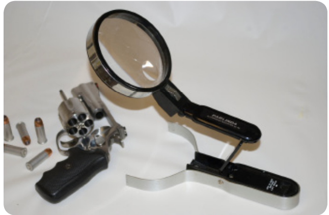
Figure 2-4: A stand magnifier allows you to work with both hands free
