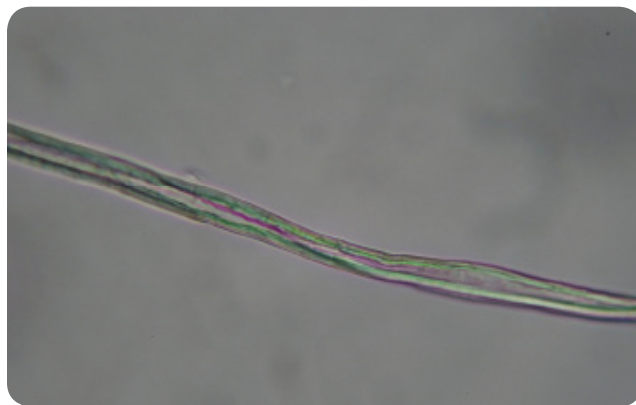
Figure II-7-11: At focus, the Becke line appears near the edge of the fiber
