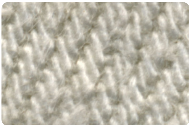
Figure II-6-3: The same fabric specimen after dye stripping
