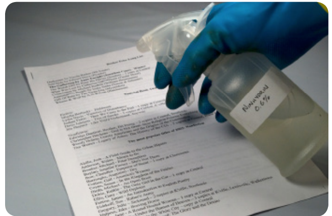
Figure IV-3-1: Spraying a specimen with ninhydrin solution
