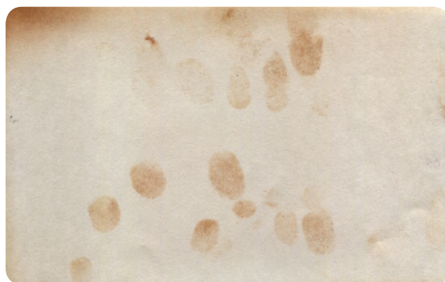
Figure IV-2-1: Fingerprints immediately after iodine fuming
