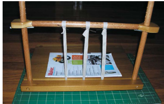
Figure 5-1 Ready to sew. Though using a stitching post is not absolutely necessary (as long as you keep a steady hand, make sure the tapes remain taut, and ensure that the signatures stay even while you sew), it does keep the work organized and easier to manipulate with the only two hands you have. If you have one available, set it up with the tapes stretched tight and spaced to match your holes.
