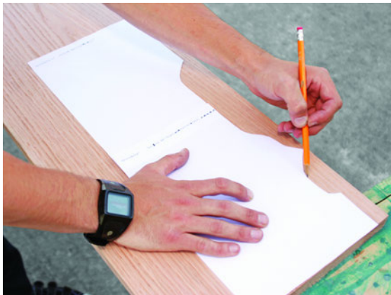
Figure 6-2 Pencil the template outline onto the wood
