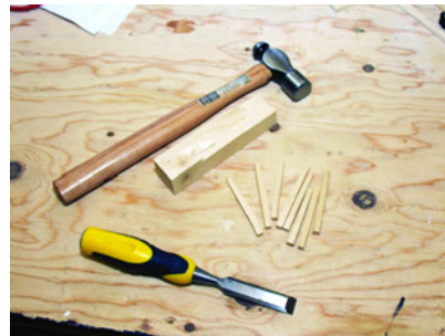
Figure 6-8 Square pegs to be fitted into the round hole you just drilled
