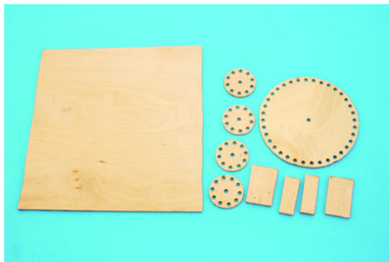
Figure 12-2 The main plywood pieces for the base, large gear, two cage gears (aka lantern gears), and one of the two towers.
