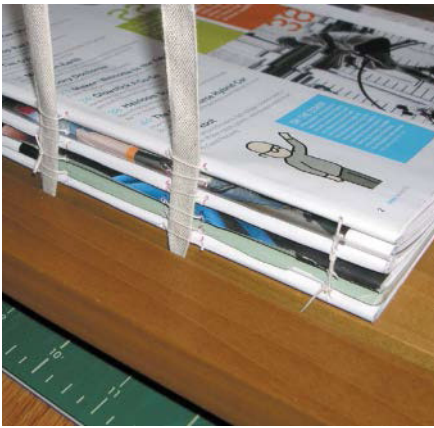
Figure 5-2 Attaching the signatures with three strips of bookbinding tape.
