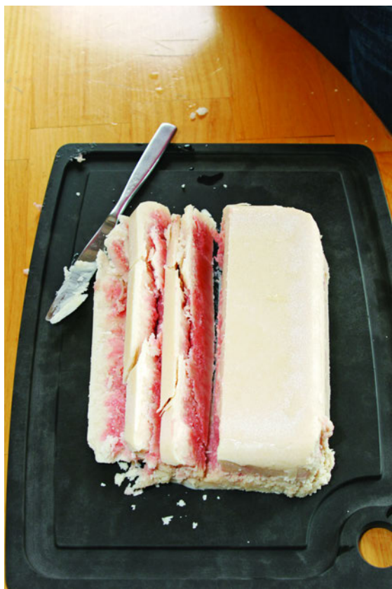
Figure 2-8 Cut the partially cured soap into desired shapes.
