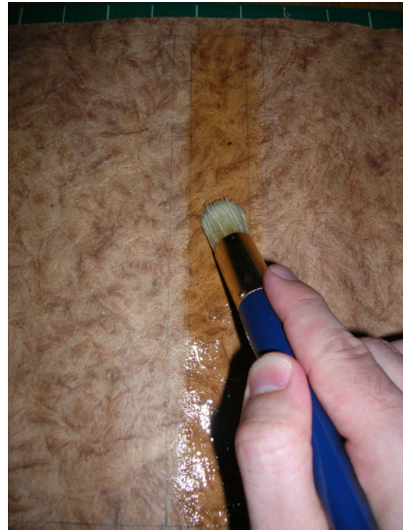
Figure 5-4 Brush the area you've marked for the front cover with glue.
