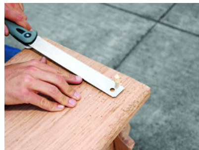
Figure 6-9 Hammer in each peg fearlessly, then saw off the remainder.
