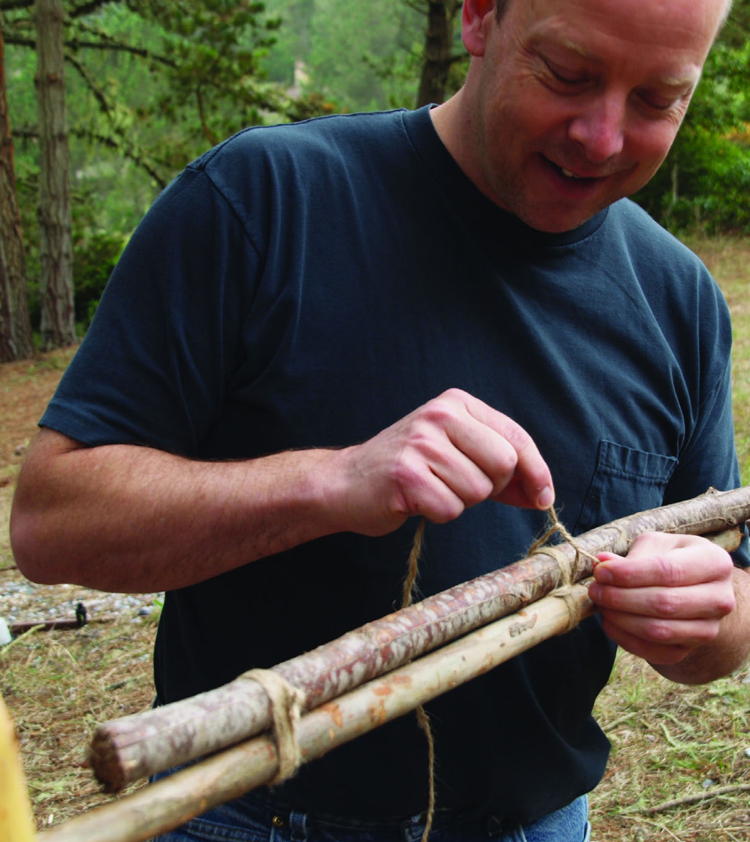
Figure 8-15 If you need to make a longer stick from two short ones, overlap and lash 'em.
