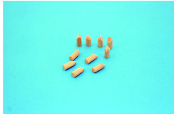
Figure 12-5 It's helpful to taper the pegs for the large gear; this will help them to mesh smoothly with the cage gears.
