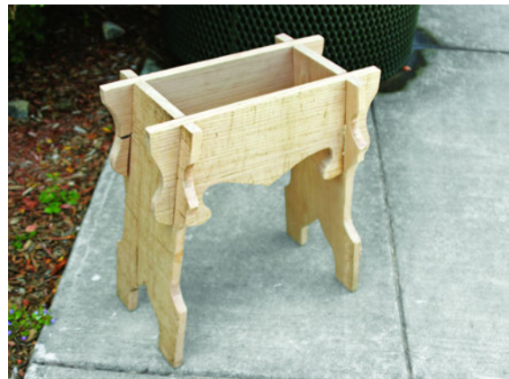
Figure 6-6 Use wood glue to hold the frame together
