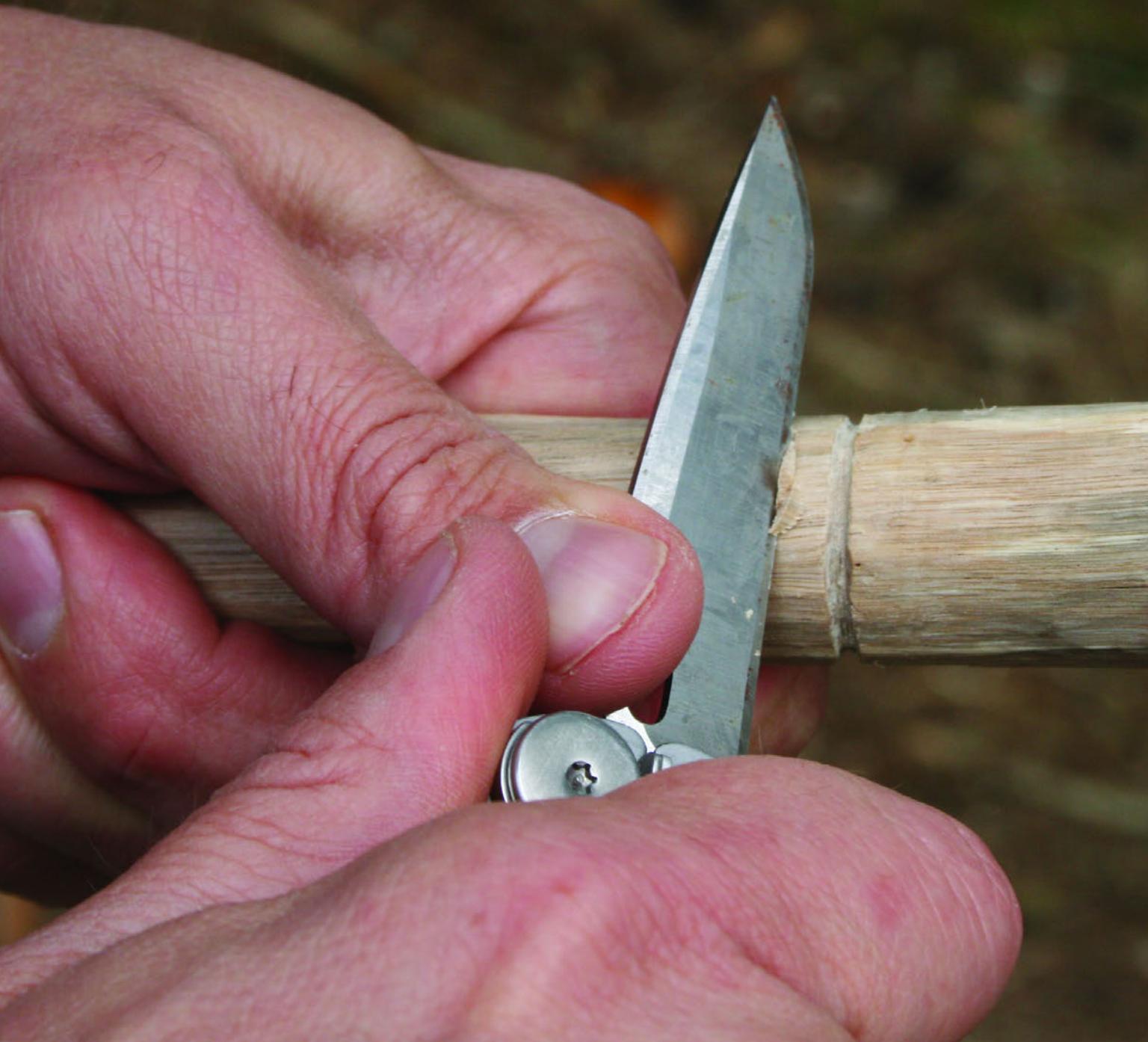
Figure 8-24 If the line slips on the wood, carve out a couple of notches to give it some purchase.
