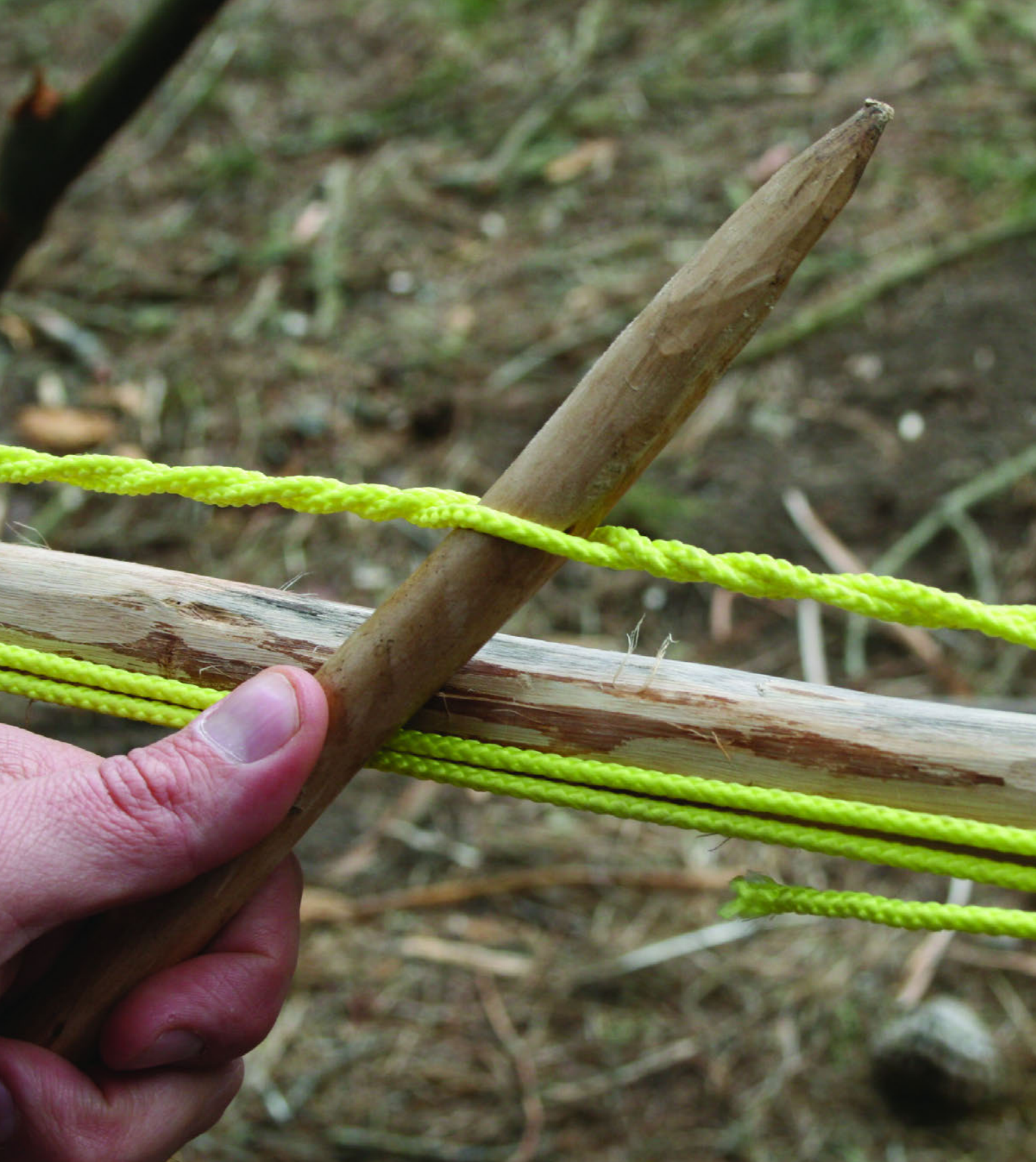
Figure 8-26 ... and a short stick make for a highly effective turnbuckle.
