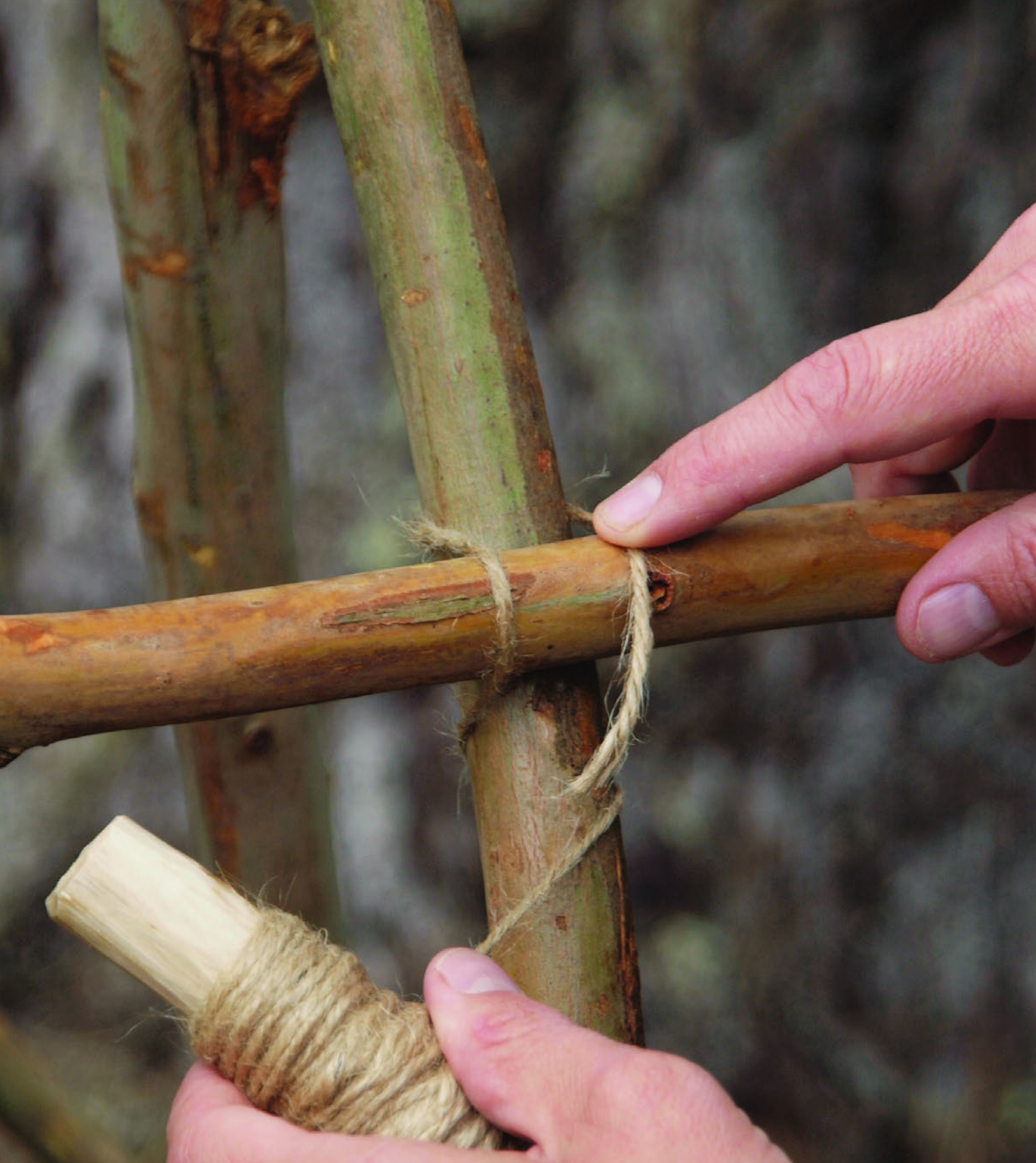
Figure 8-8 Always keep the line tight and tidy as you lay it down. Keep going until you have enough wraps.
