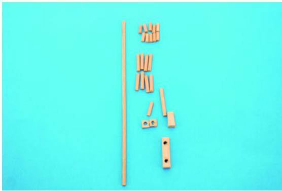
Figure 12-3 Dowels, wooden washers, and crank assembly parts. The same dowel is used to make the crankshaft and gear pegs.
