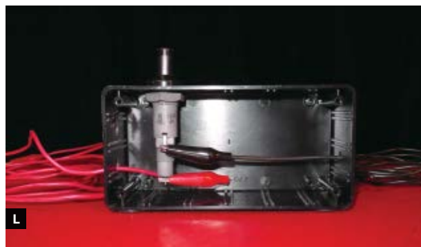
Fig. L: Ignition system: Piezo grill igniter in the project box with holes on either side to keep the leads safely separated.
