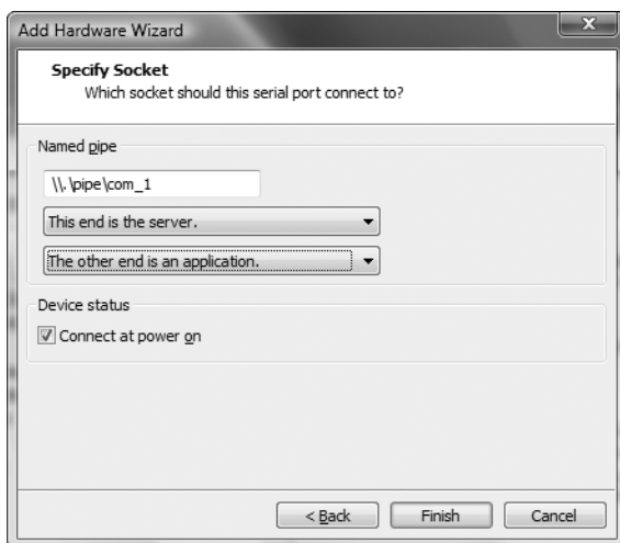
Figure B-2: Named pipe configuration
