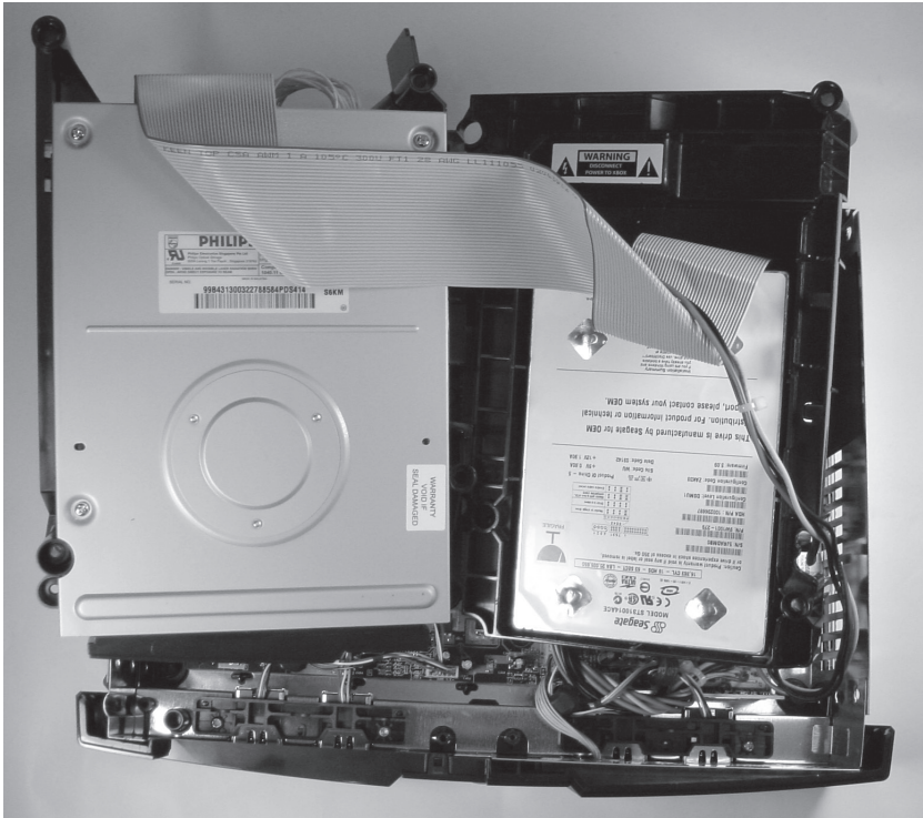
Figure 3-1: Position the disk drives so that the front edge of the motherboard is exposed.
