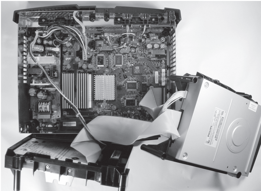
Figure 1-8: Position of the disk drives, preserving electrical connections for testing and experimentation.
