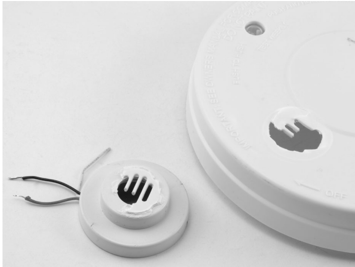
FIGURE 9-13: REMOVING THE BUZZER FROM THE SMOKE ALARM COVER
