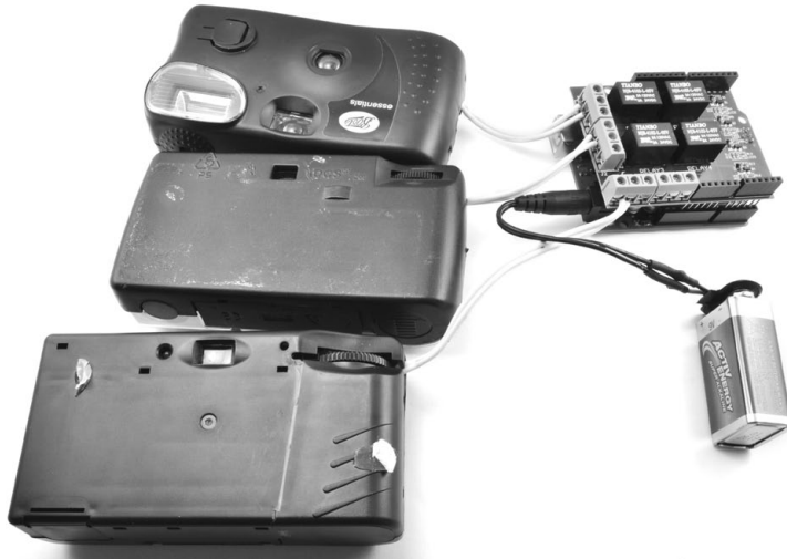
FIGURE 9-3: THE FLASH DISTRACTOR, SPREAD OUT
