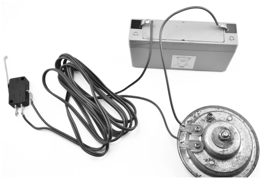
FIGURE 4-8: THE FINISHED WIRING
