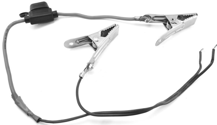
FIGURE 6-7: MAKING A BATTERY LEAD
