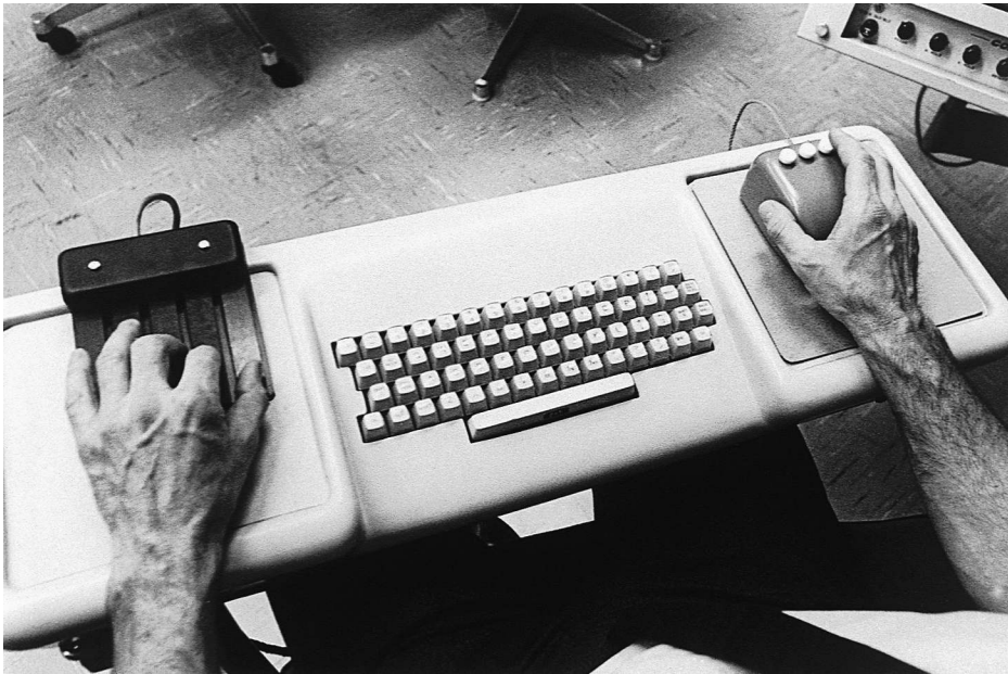
The mother of all demos: The input devices used by Douglas Engelbart at the 1968 Fall Joint Computer Conference when he put on “the mother of all demos” (Courtesy of Doug Engelbart)
