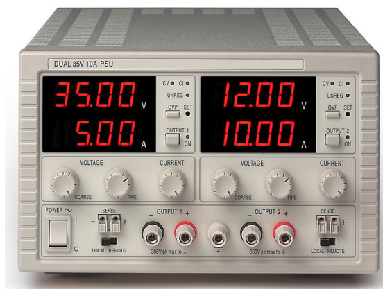
Figure 2-5. A typical bench power supply
