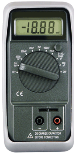
Figure 2-7. A typical capacitance meter
