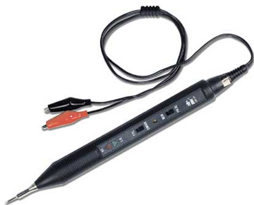
Figure 2-4. A typical logic probe
