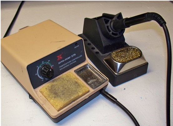
Figure 2-10. Typical temperature-controlled soldering station
