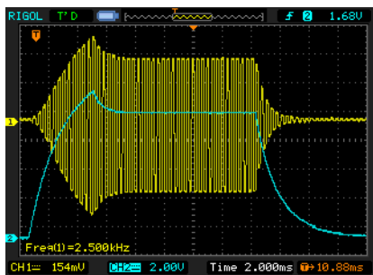
Figure 3-15. ADSR modulating a VCA
