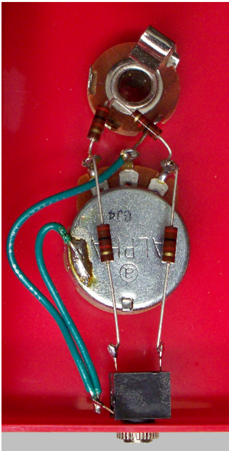
Figure 7-4. Sound card audio interface wiring (II)
