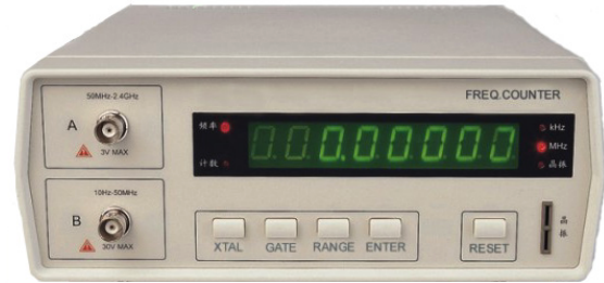
Figure 2-8. A typical frequency counter
