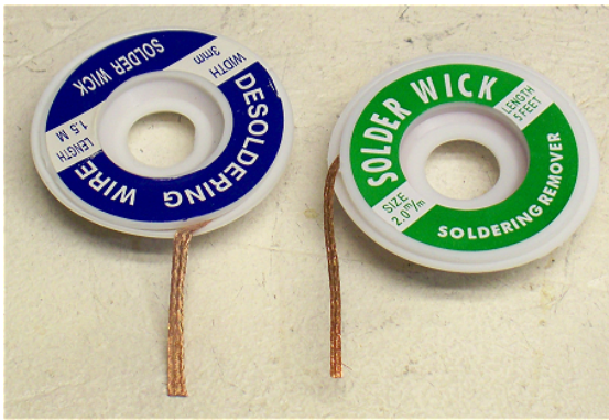
Figure 2-16. Two widths of desoldering wick
