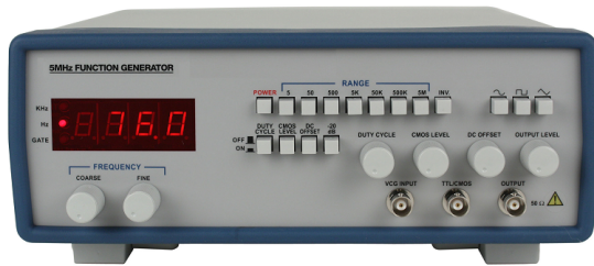
Figure 2-9. A typical function generator
