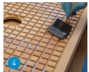
4 Sealing the MDF with wood sealer
