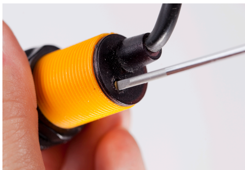
Figure 3-8. Adjusting the infrared sensor
