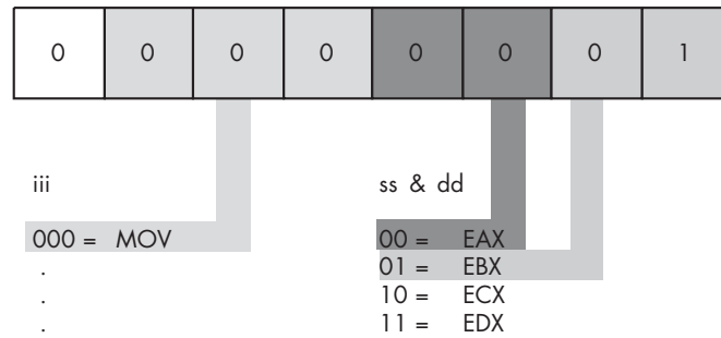
Figure 8-23: Encoding the MOV(EAX, EBX); instruction
