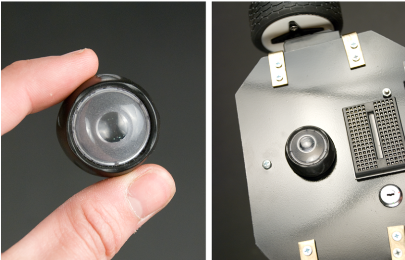
Figure 1-17. Lens glued on top of the chassis
