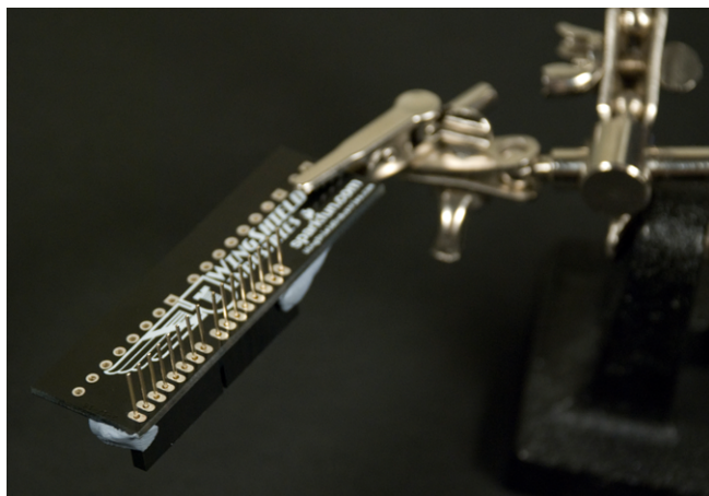
Figure A-3. Headers ready to be soldered
