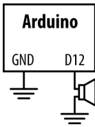
Figure 2-24. Circuit diagram for hellospeaker.pde
