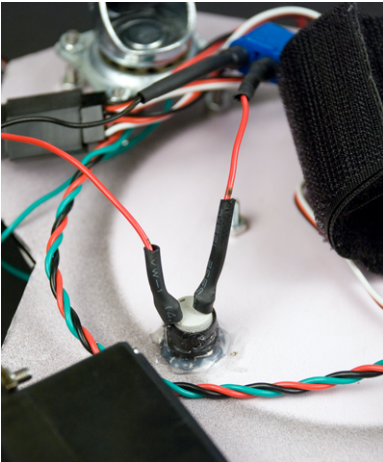
Figure 2-15. Positive wires soldered to the power switch
