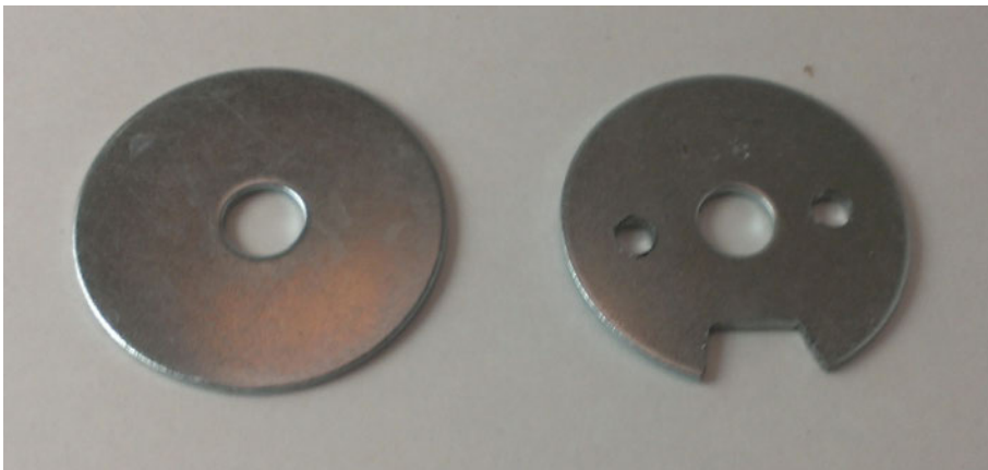
Figure 7-11. Original and modified hubcap
