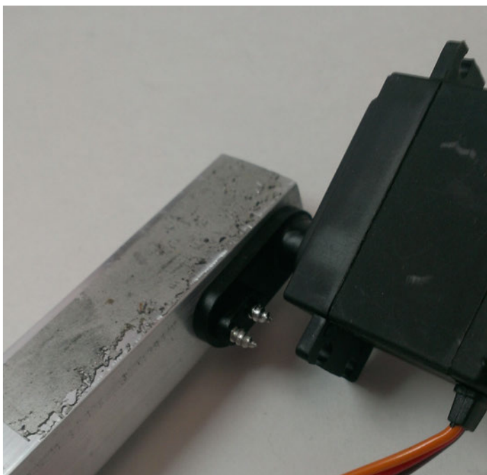
Figure 7-19. Arm attached to servo horn
