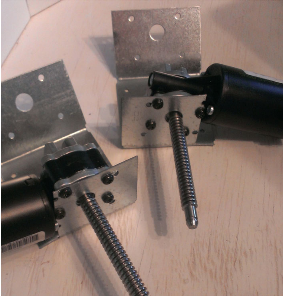
Figure 7-8. Motors attached to mounting brackets
