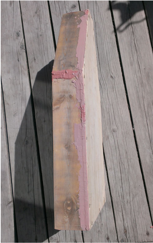
Figure 7-3. Applying filler to the gaps
