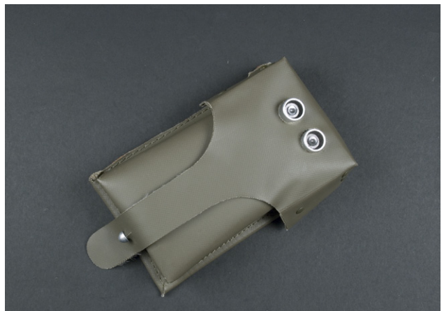
Figure 3-29. The ultrasonic sensor in place
