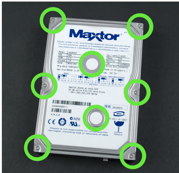
Figure 8-26. Locations of screws
