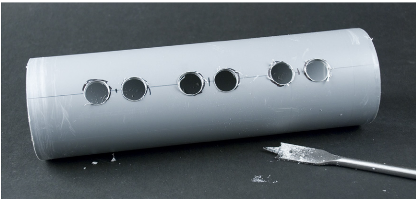
Figure 5-29. The 16mm holes for the sensors
