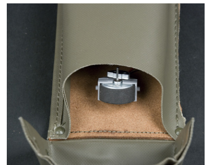
Figure 3-25. The vibration motor in place
