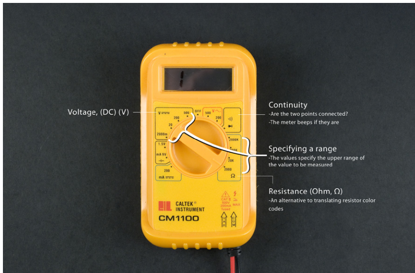
Figure 1-26. The most common functions of a multimeter
