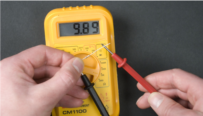
Figure 5-6. Measuring resistance with a multimeter
