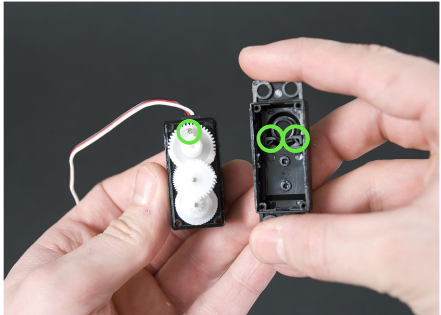
Figure 8-9. Obstructions that block rotation
