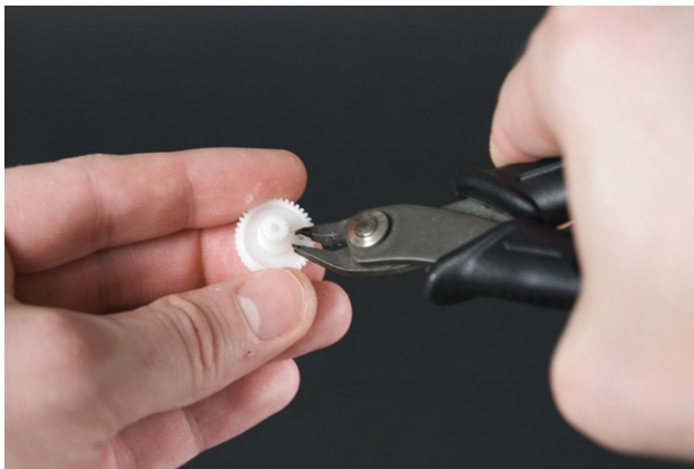
Figure 8-10. Cutting off the obstructions
