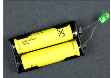
Figure 1-28. Simple closed circuit powering an LED
