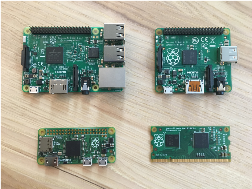
Figure 1-1. There are many versions of the Pi, and here are a few (clockwise from top left): Raspberry Pi 3 Model B, Raspberry Pi 1 Model A+, Raspberry Pi Compute Module, and Raspberry Pi Zero. As of February 2016, Raspberry Pi 3 Model B is the latest mainline Raspberry Pi.
