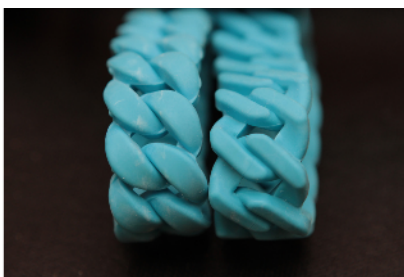
Figure 6-36. Chain bracelets repurposed as rover treads
