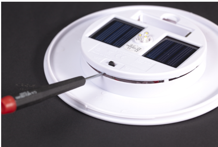
Figure 7-29. Pry the bottom cover lid off
