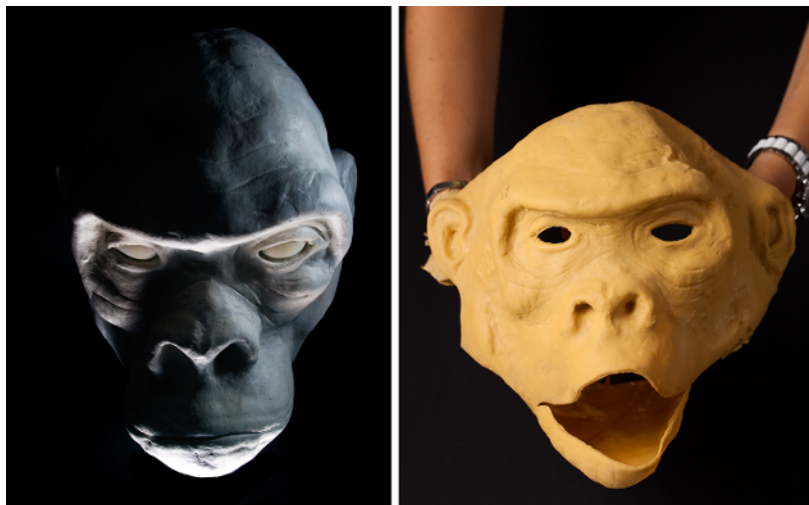
Figure P-5. Base model for animatronic gorilla head and latex skin made from it.
