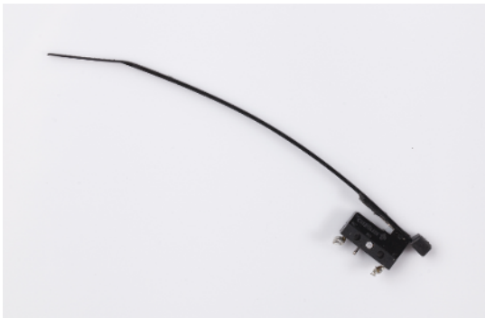
Figure 5-7. Feeler antenna from microswitch
