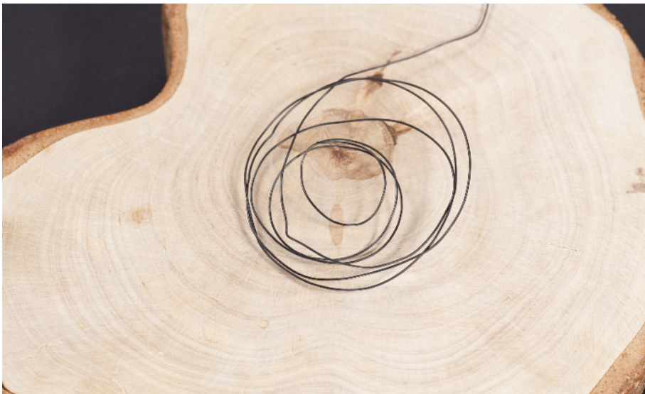
Figure 5-16. Touch wire spiral, hidden from user
