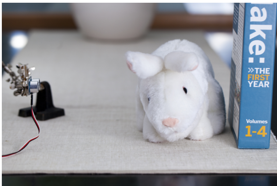
Figure 3-7. Testing ping sensor with a soft object
