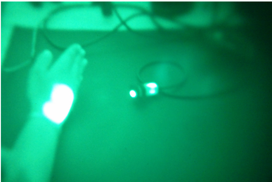
Figure 3-13. The IR sensor seen through night-vision goggles
