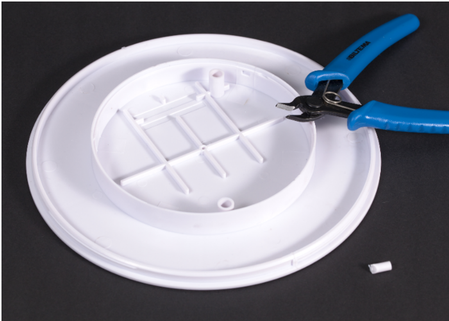
Figure 7-31. Cut the little stick off from the center
