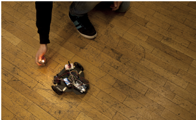
Figure 7-2. Flame-following robot prototype (robot workshop in Austria)
