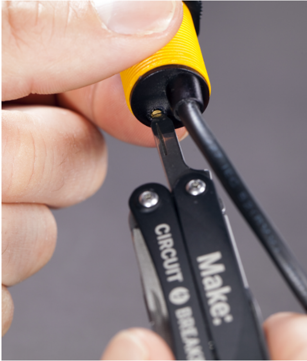
Figure 3-9. You can adjust the distance to which the sensor detects obstacles
