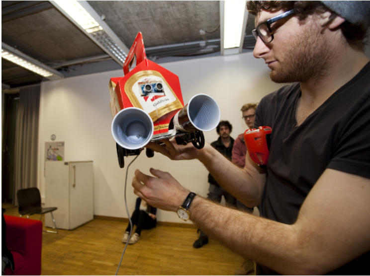
Figure 7-12. Photoresistors inside plastic cup blinkers (robot workshop in Austria)
