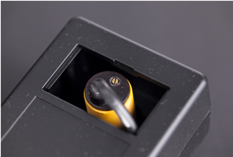
Figure 3-23. From the back of the chassis, you can adjust the distance screw
