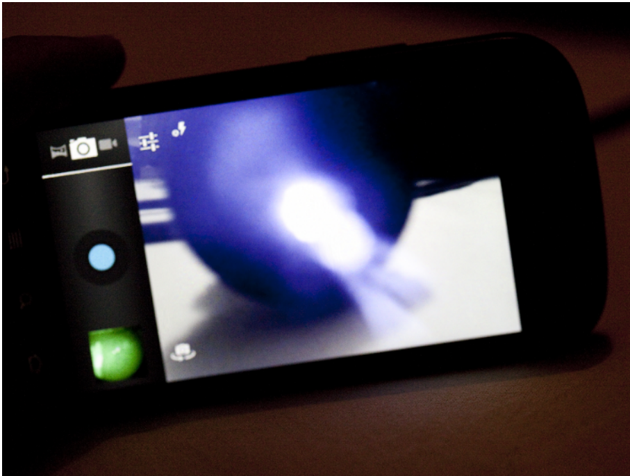
Figure 3-12. How a phone's camera sees IR sensors
