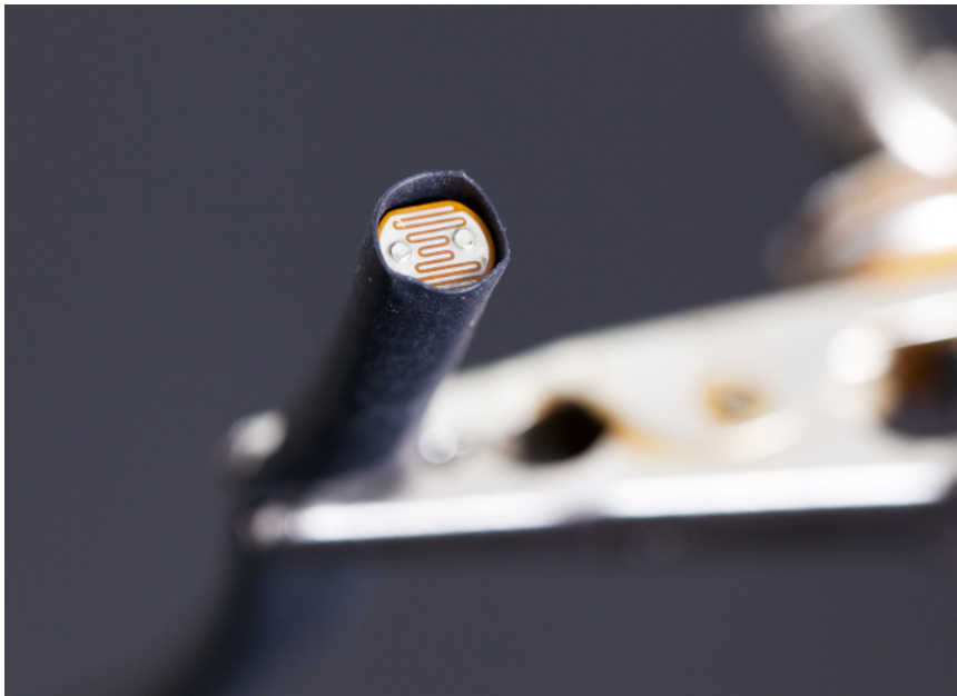
Figure 7-11. Preventing light from reaching the sensor
