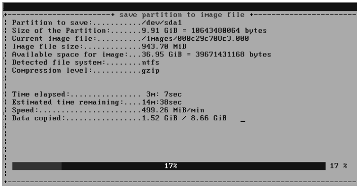
Figure 7-13: Transferring the client’s disk image
