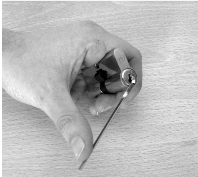
Figure 5.12 Lock with torque wrench inserted.
